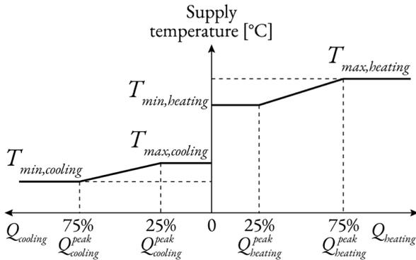
**Figure 2: Demand-based temperature control curves.**
