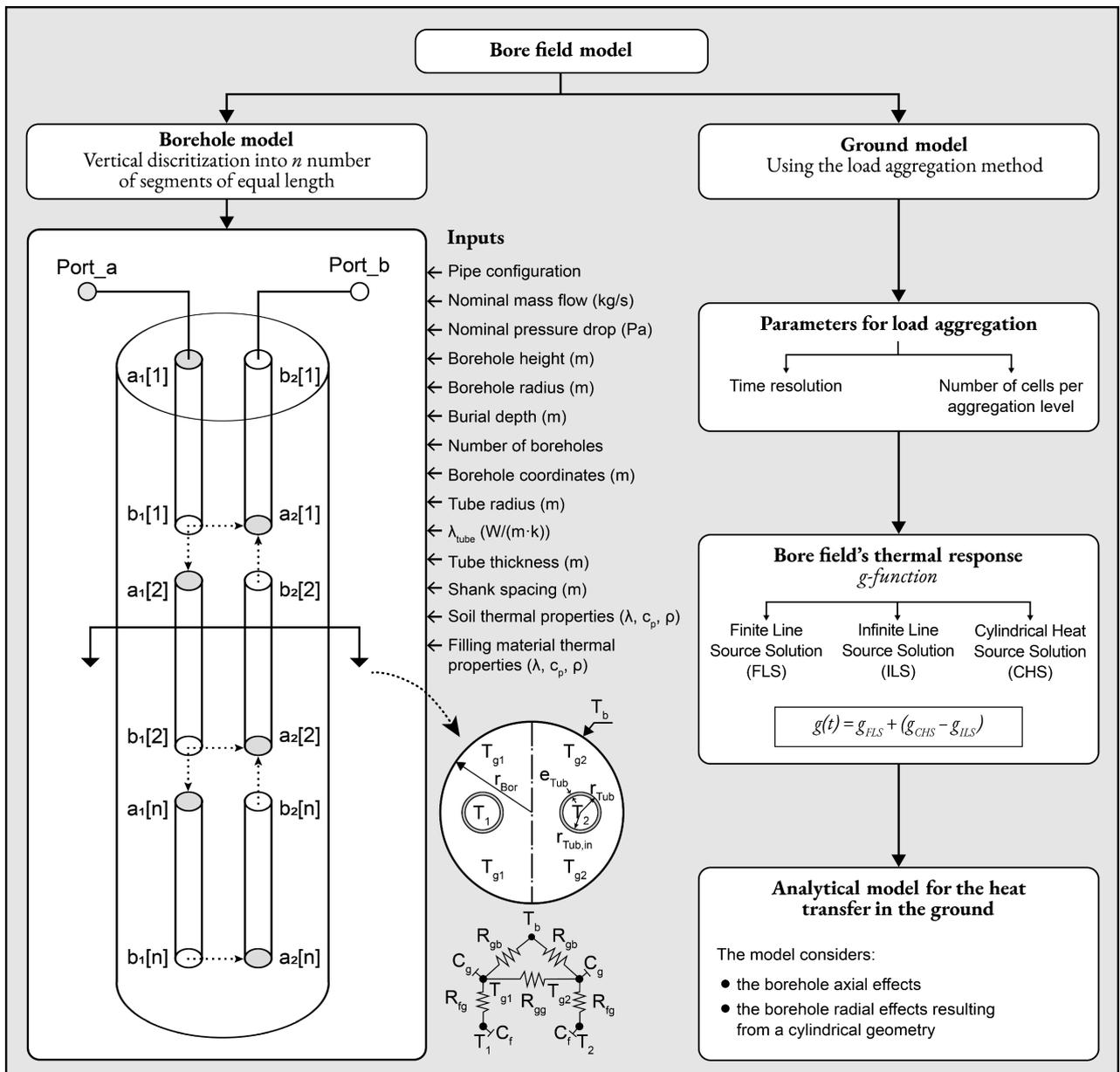
**Figure 4: Bore field model structure.** The borehole model is shown for a single U-tube configuration where heat extraction from the ground is indicated by a flow direction from port\_a to port\_b. The delta-circuit of thermal resistances is adopted from Bauer et al. (2011).
